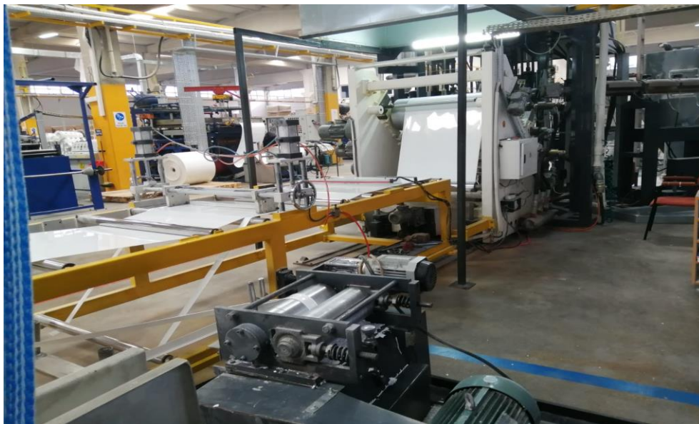
Figure 1. The plastic extrusion line that will be optimized
